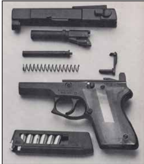
Here's the ASP broken down to its basic parts. Silhouette of the Guttersnipe sight is apparent and the transparent grips allow a quick look at your ammo supply. Special grips will not yellow with age.
