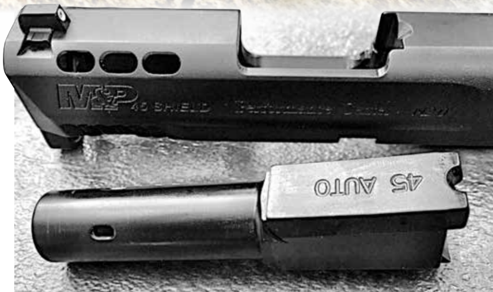
The ported barrel and slide: The simple dispersion of gases helps us by reducing felt-recoil and muzzle-flip. It works, too!
