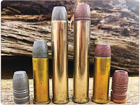
Tank's favorite molds for the .444 Marlin — LBT 330-grain LFNDCGC at left and MP Molds 300-grain HP on right. Both molds work wonderfully in .44 Mag too!
