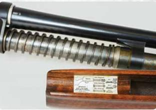
In the A5/M11, Browning incorporated a clever series of fouling-insensitive friction rings around the magazine tube to adjust the gun for differing loads.
