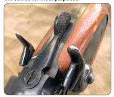
Pushing the top lever to the left will allow the gun to break open for loading and unloading.
