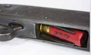
The Model 37 both loads and ejects through the bottom of the receiver, with no opening on top or sides to allow in water, dirt or garbage into the bowels of the receiver.
