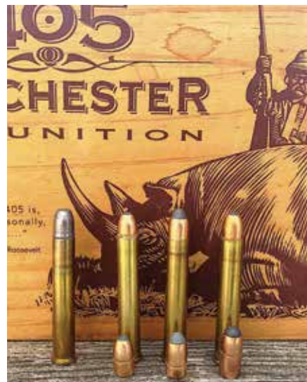
Here's the .405 Winchester line-up (from left to right) — a sized-down RCBS 0.417" cast bullet, and Northern Precision bullets 225-, 265-, and 325-grain.
