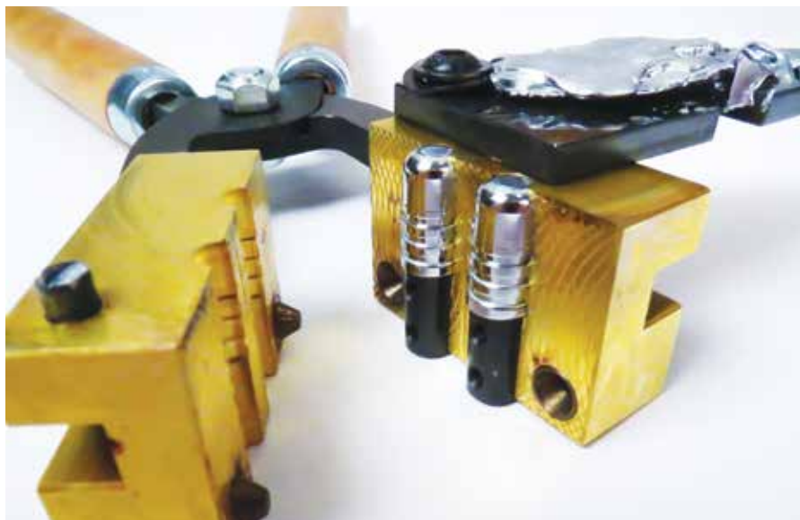
One of Duke's most recent molds came from Slovenia. It's a multiple cavity .41 Colt hollowpoint design weighing 190 grains.
