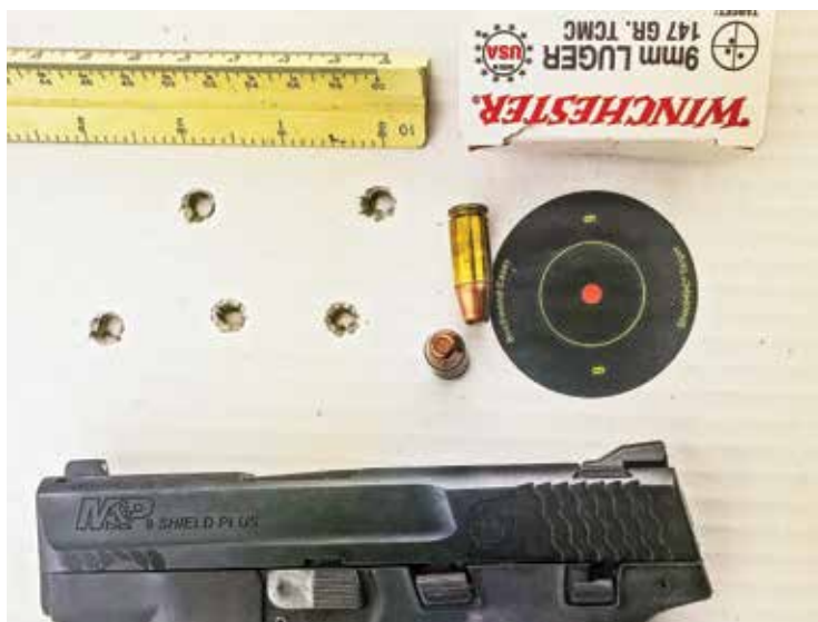
The 25-yard bench performance was good for such a small pistol (above). Don’t let others fool you with short-range sub-compact tests; bad guys don’t move closer because you’ve got a tiny pistol! Surprisingly, Winchester 147-grain FMJ gave the best 25-yard accuracy test (below).
