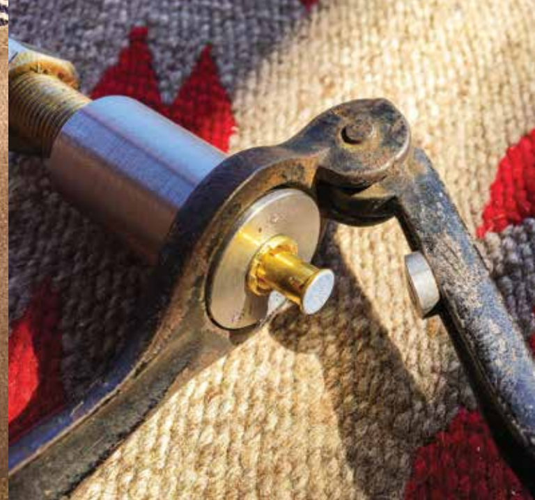
Dennis Heckman enjoys re-purposing old reloading gear like this old shotgun primer reloading tool, used to press the power load into the case.
