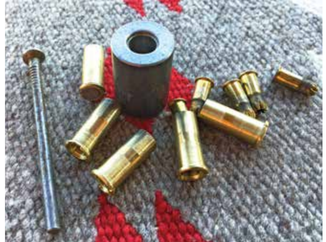
In many ways, Heckman's tools mimic the Lee Hand Loader sets. A common nail is used to punch out the spent power loads.
