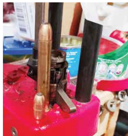
Tank's Lee Classic Turret press, with Hornady dies was used for all handloads with excellent results.
