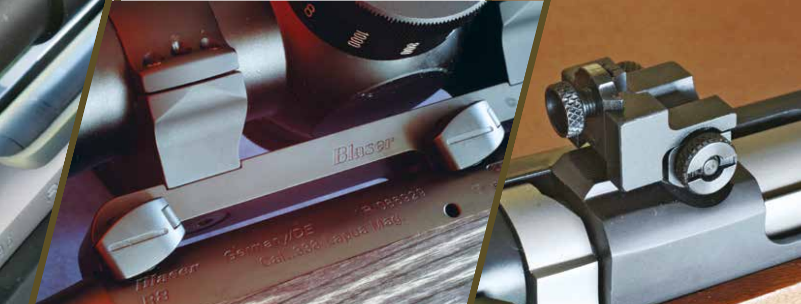
Folding tabs on Blaser's thumb-screws (above, left) dodge anything that might snare them. Hand-tightened, they defy even magnum recoil. Wayne found return to zero adequate for 600-yard hits on an 8" target! This excellent aperture sight by New England Custom Gun (above, right) quickly replaces a QD ring in the machined pockets of a Ruger 77 receiver.
