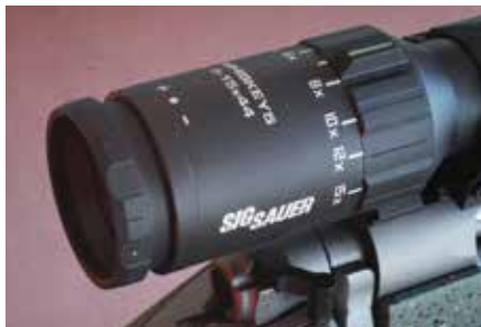
Internal design and ocular lenses — not the objectives — determine FOV, by angular and linear measure.
