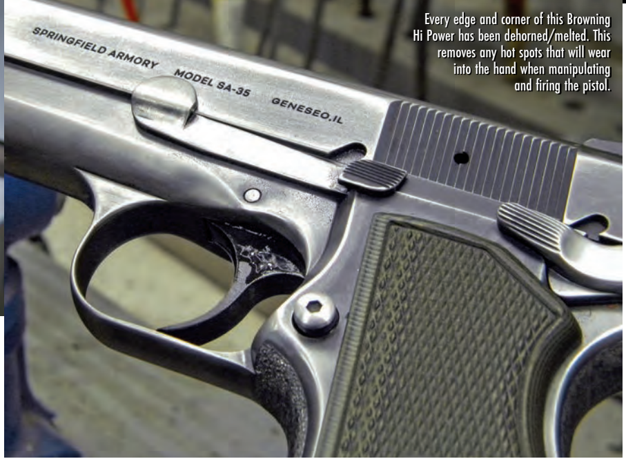
Not all melting is about how you grip the pistol. Putting a smooth radius on the front of the barrel or slide makes it easier to holster smoothly.
