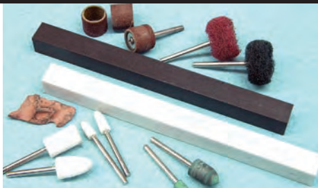
Tools of the trade include hones, various polishing pads and, for more aggressive metal removal, sanding drums and hard rubber polishing wheels.
