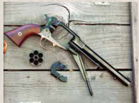
Remington Percussion Pistols can be changed to cartridge firing with the addition of a conversion cylinder.
