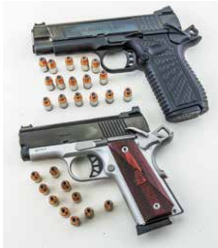
Here are 1911s built from the ground up for the 9x19: the double stack Wilson SFT9 (top) and single stack Springfield EMP. Photo by the author
