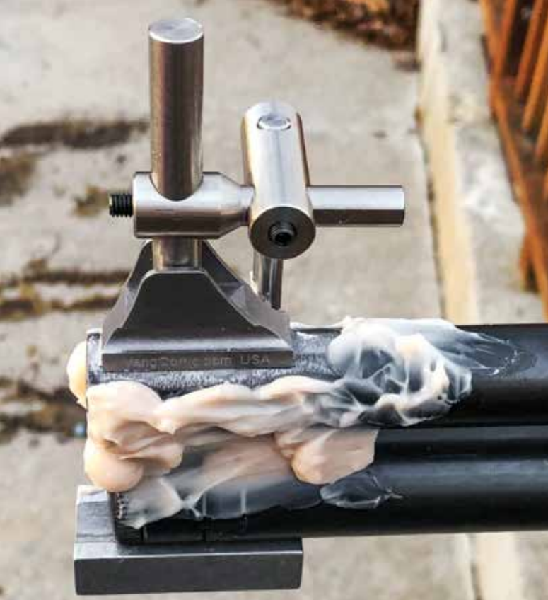
The front sight (above) jugged up and ready for the oxyacetylene torch. The receiver (below) was spotted using a 3/32" ball end mill for the sight base holes then tapped #8-40. This is an uncommon size but easy to find on Amazon.
