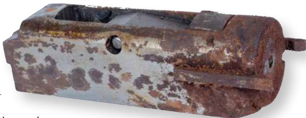
Jeremy's beloved Mossberg 500 was nearly reduced to scrap after being shot with corrosive ammo and accidentally left to rust. Fortunately, it's back to fighting trim and with a few improvements!
