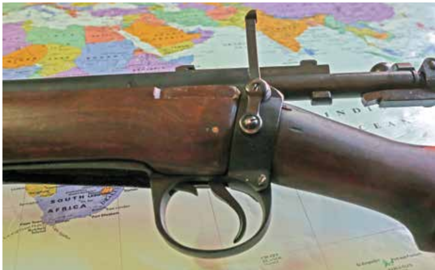
The MLE (Magazine, Lee Enfield) had a barrel-mounted open rear sight and also this “volley sight” for shooting at extreme ranges, out to 2,800 yards.
