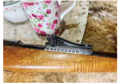
The precision craftsmanship of the Mauser ladder-rear-sight by the long-dead builders is simply amazing.
