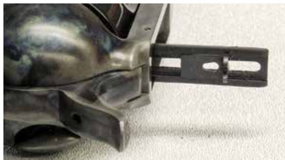
The rear sight of the Uberti Flat-Top frame shown raised out of its mortise.
