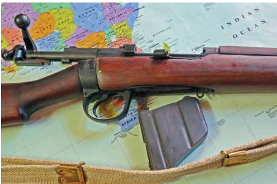
One of James Paris Lee’s innovations was the double-stack detachable magazine. The rear locking lugs of the bolt meant bolt throw needed to be just a bit longer than the .303 cartridge, making for fast cycling.
