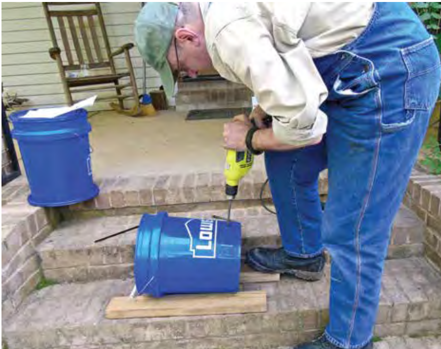
The hole for the spigot is located 2" from the bottom of the collection bucket. This allows clearance for the tap. A standard spade bit bores the hole painlessly.
