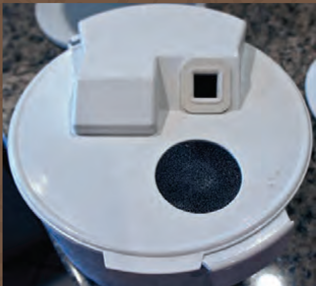
This is the top of the storage container located beneath the grinder. Make sure the seal between the machine and the storage container is sealed or you will end up with a flour cloud all over the kitchen.
