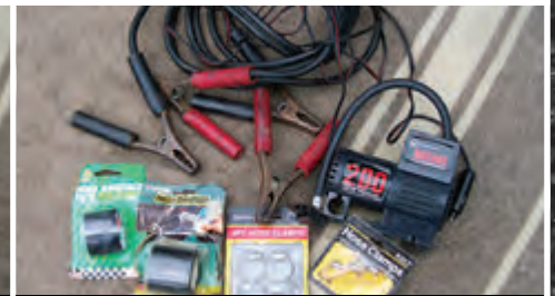
A good set of jumper cables is a must, along with hose bandages for blown radiator hoses, and an air compressor to pump up flat tires.
