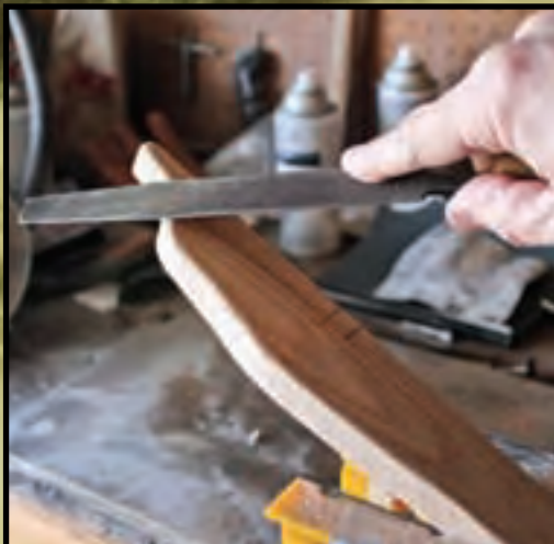
Sketch the outline of the stock on a piece of 1X3 red oak (above). Cut the stock out with a bandsaw or coping saw (left). Use files and sandpaper to smooth the stock to finished form (below).
