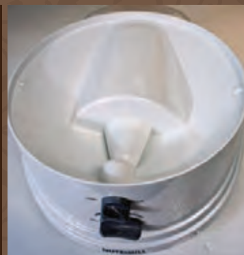
This is the top of the storage container located beneath the grinder. Make sure the seal between the machine and the storage container is sealed or you will end up with a flour cloud all over the kitchen.
