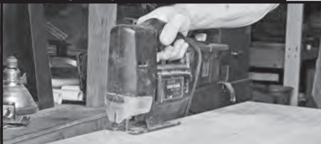
Power saw: Cutting plywood to fit windows properly is best done with power saws, and they work best with — power. Since blackouts often accompany disaster situations, it's best to plan ahead.
