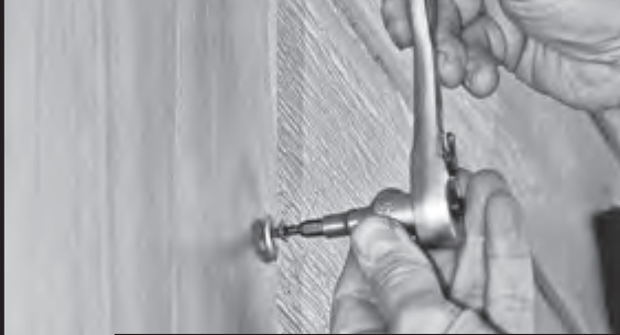
Socket as a screwdriver: If the power goes out, a socket wrench with a 1/4" socket can be used as an improvised power screwdriver.
