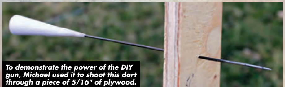
The spring steel/paper cone dart achieved a velocity of 172.2 fps.
