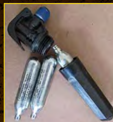
The CO 2 bicycle tire inflator doesn't put out massive flow, however, a few CO 2 cylinders can encourage a slow leaking tire back to the ATV.
