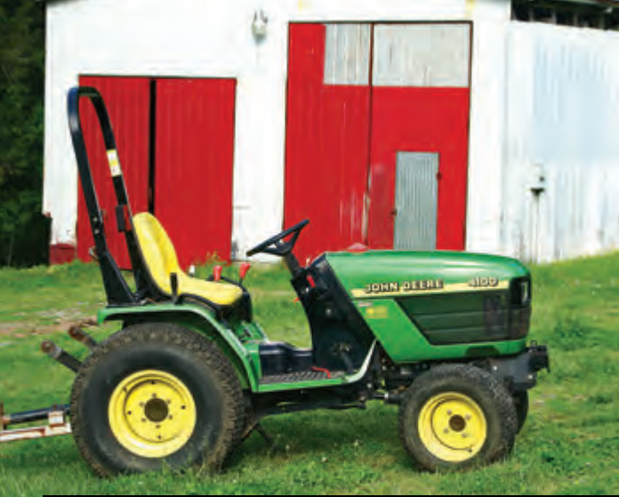
Our 20-HP tractor with power take off and a 3-point hitch. It does everything on our 30 acres that we need.
