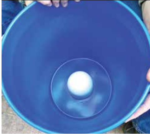
Once the filter is in place the rest of the device just snaps together. Ceramic filters are brittle and should be handled carefully.
