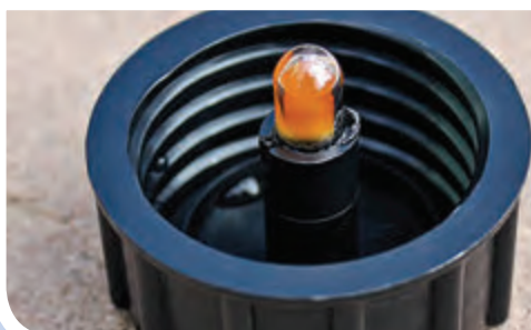
A WAPI (water pasteurization indicator) is a reusable temperature-sensitive vial containing wax that melts at 149 degrees F, providing a definitive indicator that pasteurization temperature has been reached. It is built into the AquaPak's cap.
