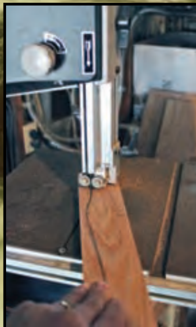
Sketch the outline of the stock on a piece of 1X3 red oak (above). Cut the stock out with a bandsaw or coping saw (left). Use files and sandpaper to smooth the stock to finished form (below).
