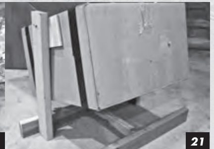
(19) When the panels are raised and joined at the edges they provide increased surface area and the ideal angle to reflect sunlight into the oven. (20) The oven's window in place. The fit should be snug to retain heat. (21) To allow the oven to be free standing and easily oriented toward the sun, the author made this simple frame from scrap 2x4s. (22) Wing nuts and washers on the 1/4" carriage bolts allow the angle of the oven to be easily adjusted to maximize its exposure to the sun. (23) The finished solar oven — ready for a "test drive." (24) The test conditions for the oven were partly cloudy skies and air temperatures that ranged from just above freezing to about 47 degrees F.
