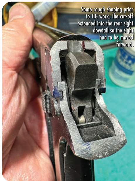
Extensive machine and hand work teased the Mini-1911 into existence. Look carefully and you can see the weld repair marks and bevels and such that were done.
