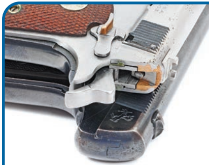
Cosmetic work still needs doing here but this shows the rough relationship to the original shape. Note how the rear sight is moved well forward. The hammer still needs checkering here.
