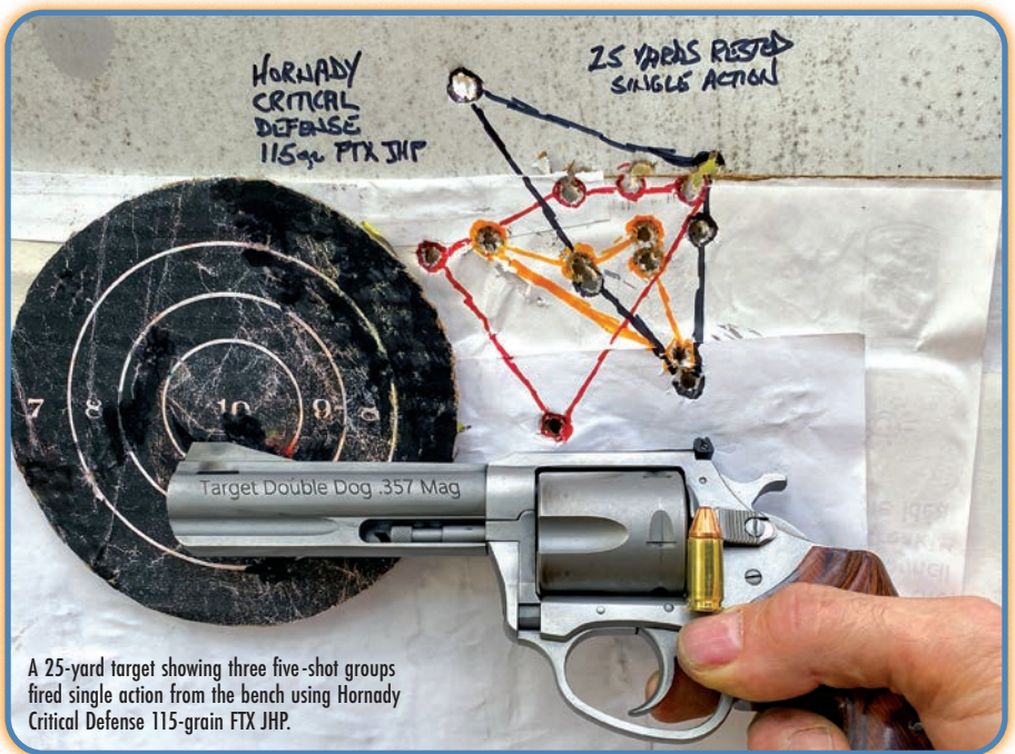
Note how the grip is flat across the front strap. I found this design feature helped stabilize the pistol in my grasp, especially in one-handed single-action and double-action shooting.
