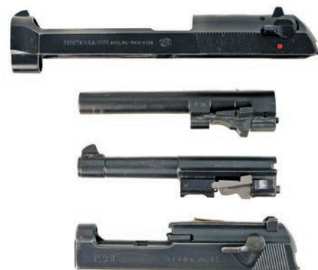
The locking system of the Beretta M9 (top) was copied from that of the German wartime Walther P38.
