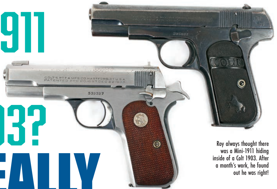
Extensive machine and hand work teased the Mini-1911 into existence. Look carefully and you can see the weld repair marks and bevels and such that were done.
