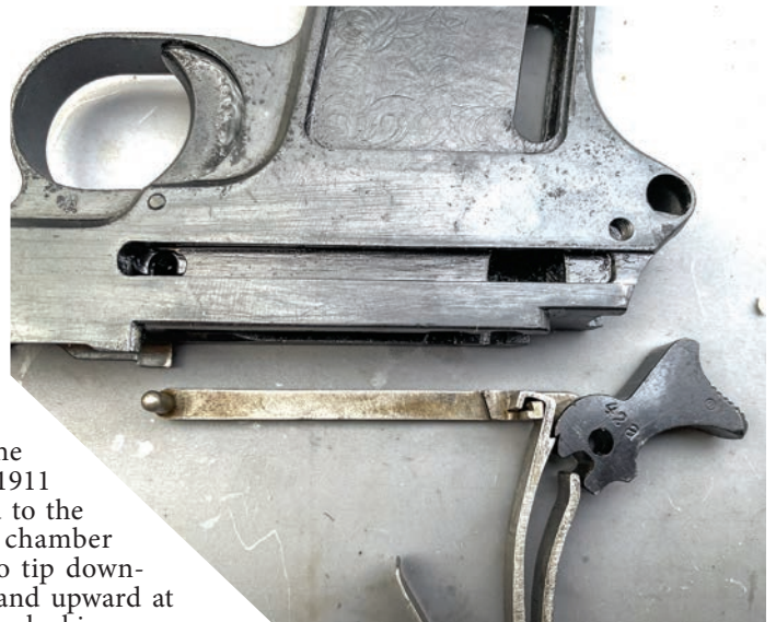
Below: Trigger bar, sear spring, hammer and hammer spring arranged to show their relationship to each other when installed in the frame (above). Note how the sear spring is also the sear.
