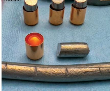
Lindsey scored the lead wire he purchased from Rotometals and stuck them into the 0.45" x 0.580" jackets from Center X Bullets.
