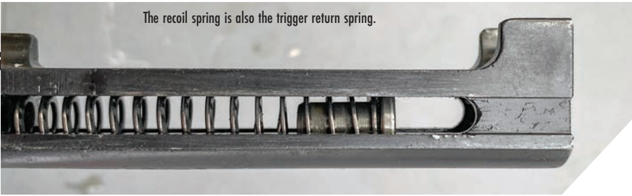
The frame has slots in the sides at the front and rear that mate with rails on the slide, making for a rigid connection.
