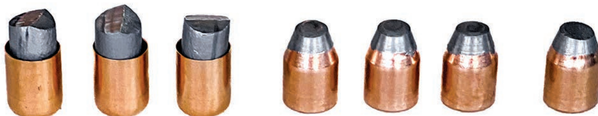
The lead cores in the jackets sort of look like lipsticks before the lead is pushed into the jacket. The bullets on the right are some of the first swaged bullets Lindsey made using this method.
