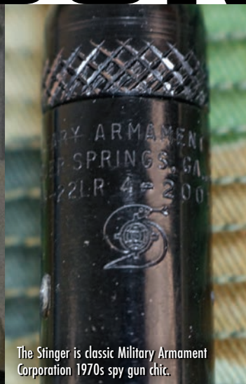
Cocking the Stinger involves unthreading the base cap and pulling it back until the striker catches.
