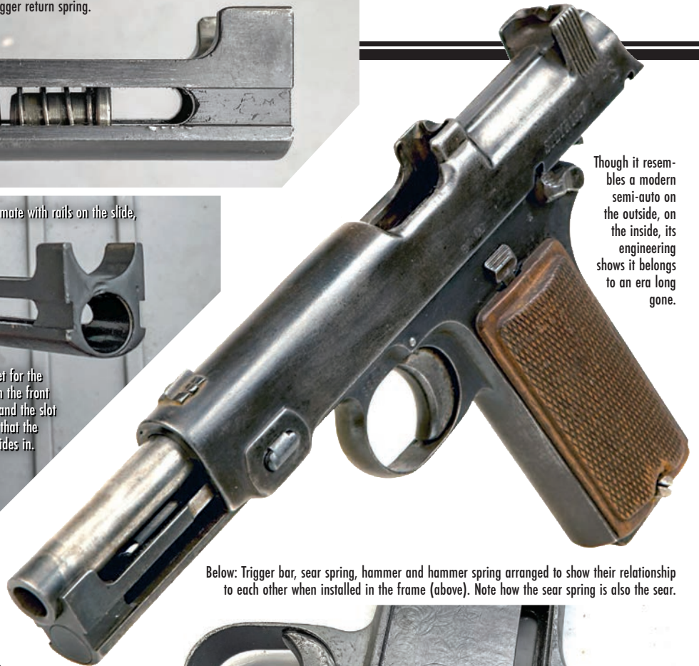
The recoil spring is also the trigger return spring.
