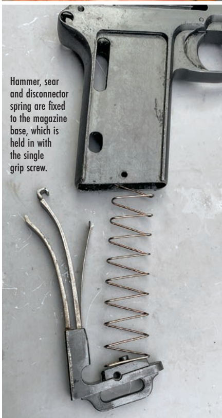
A very efficient design, the pistol has only 32 parts, all of them shown here.
